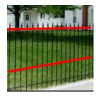
This fence could be retrofit by removing the finials (pointed tops) and adding a cross member at the top and the two foot mark.
