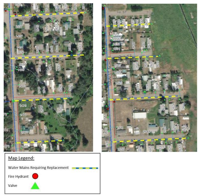
The replacement main will be constructed in the same location and water services will be renewed as a part of the scope of work. The RDOS will work with consultants and contractors to minimize the disruption to residents during construction.
