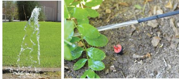
*broken sprinkler head & missing drip emitter*
