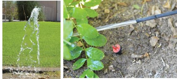
*broken sprinkler head & missing drip emitter*
