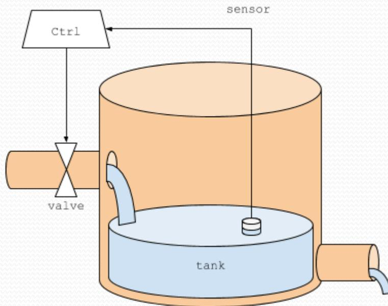
A lift station – moving influent up and along the pipes to and in the treatment process
