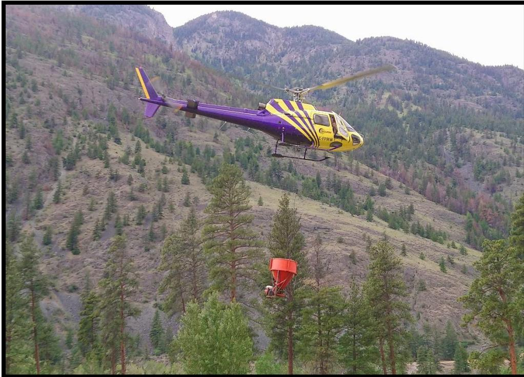
Figure 2.3: Treatment Hopper under the Helicopter
