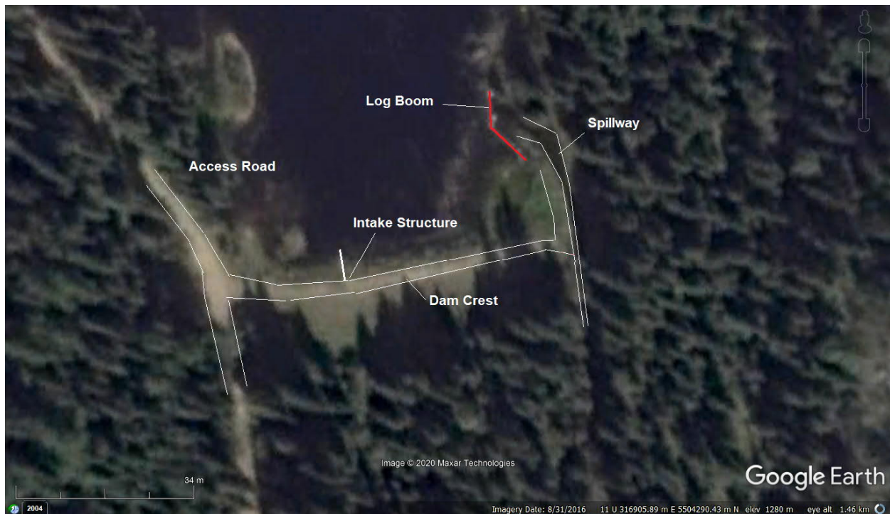
Figure 2-2: Elinor Lake South Dam Major Component Layout
