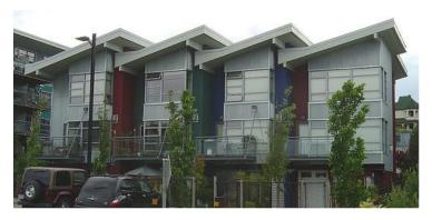
e) Medium density residential buildings greater than three storeys in height should have the fourth and any higher floors stepped back a minimum of 2.1 metres to reduce the apparent building height and bulk.
