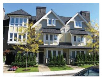
b) The ground floor of all medium density residential buildings should be raised a minimum of 0.6 m above adjacent grade to create a clear separation of public and private space, with raised front porches or stoops for all ground floor units.
