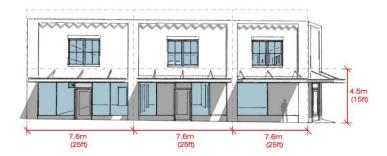
h) Where a single, larger format commercial use exceeds a frontage width of 15.0 metres, the principal street frontage should be lined with smaller individual commercial retail units (CRUs) that screen this larger commercial use, with a narrower portion of the main use visible to the street.
