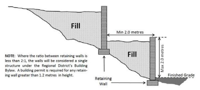
Figure 7.28.4: Retaining Wall Illustration
