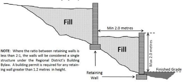
Figure 7.25.4: Retaining Wall Illustration
