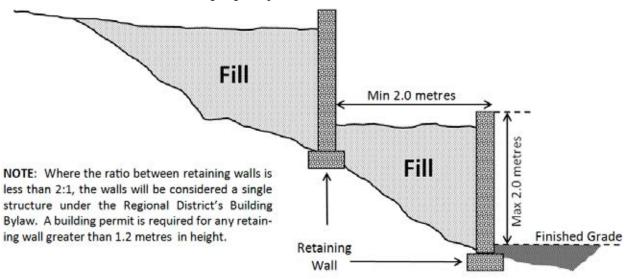
Figure 7.25.4: Retaining Wall Illustration
