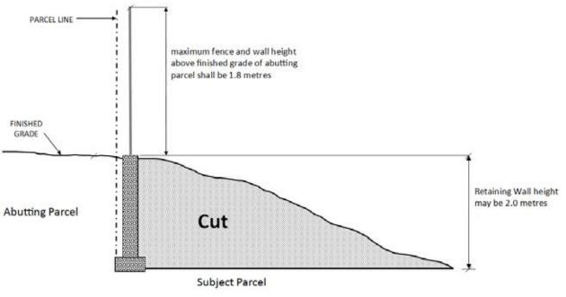
Figure 7.25.5: Retaining Wall in a Setback Illustration
