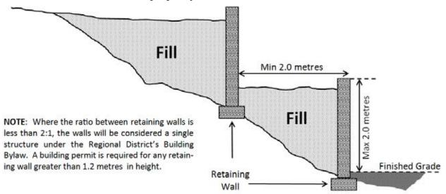
Figure 7.25.4: Retaining Wall Illustration
