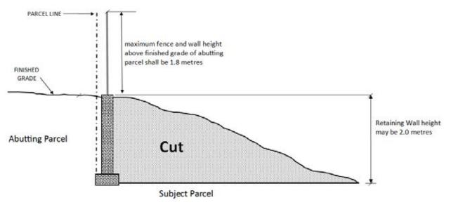
Figure 7.25.5: Retaining Wall in a Setback Illustration
