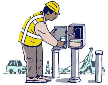
In addition to the weekly bacteriological samples, field tests are conducted for free chlorine residuals, temperature, pH, conductivity and turbidity.
