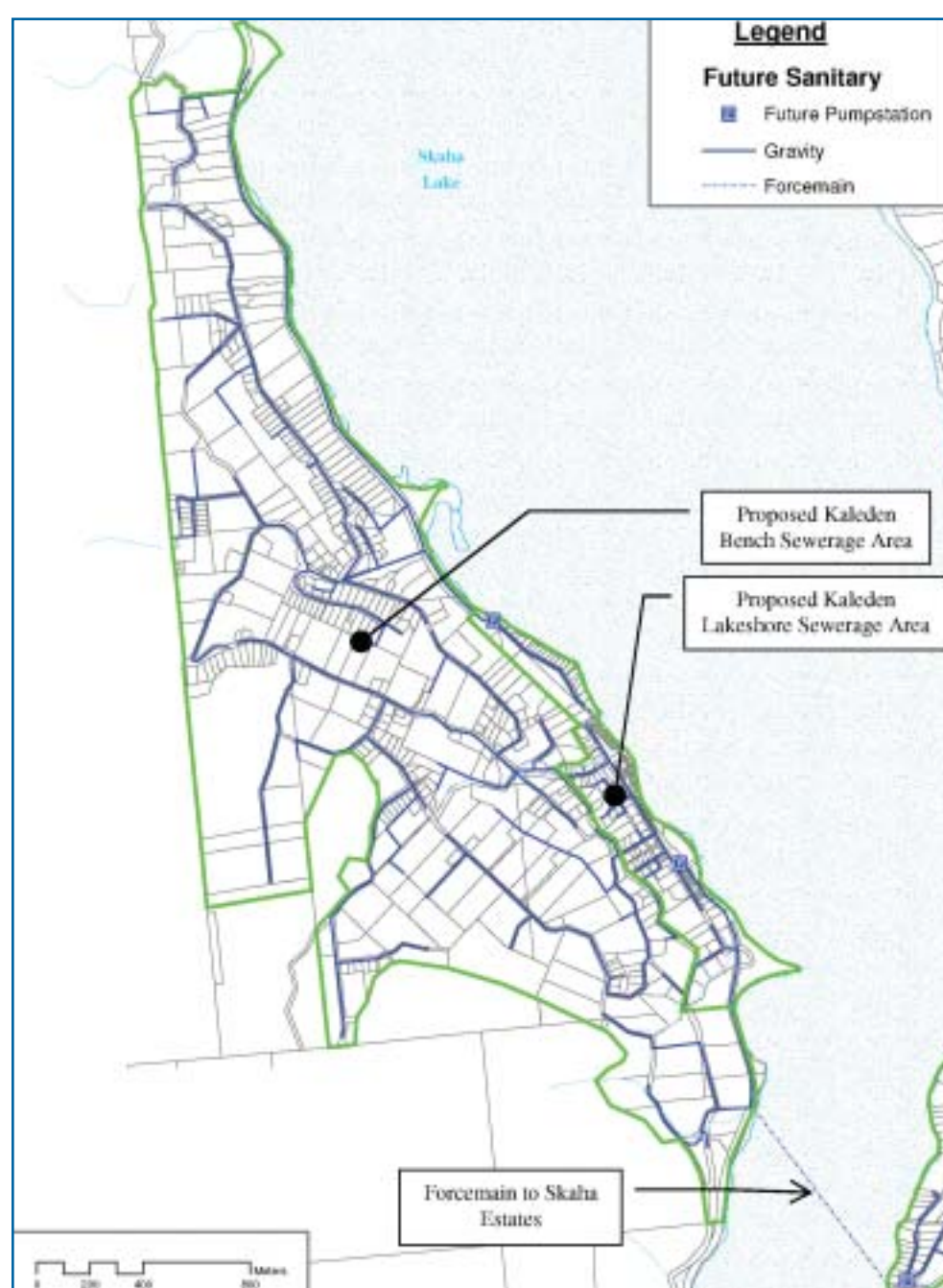
Proposed future Kaleden sewerage system
