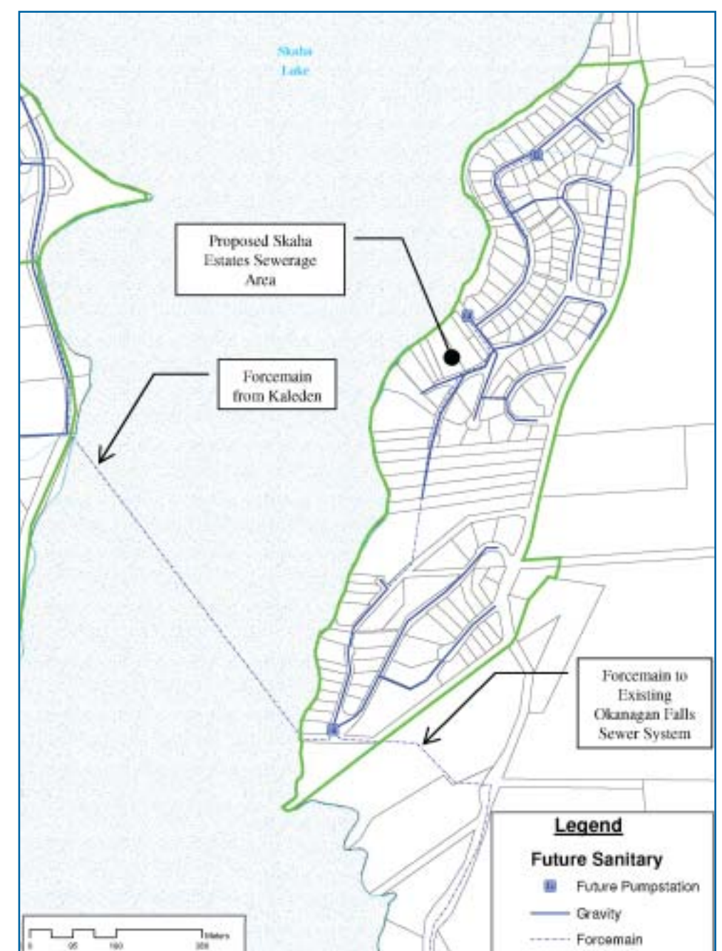
Proposed future Skaha Estates sewerage system
