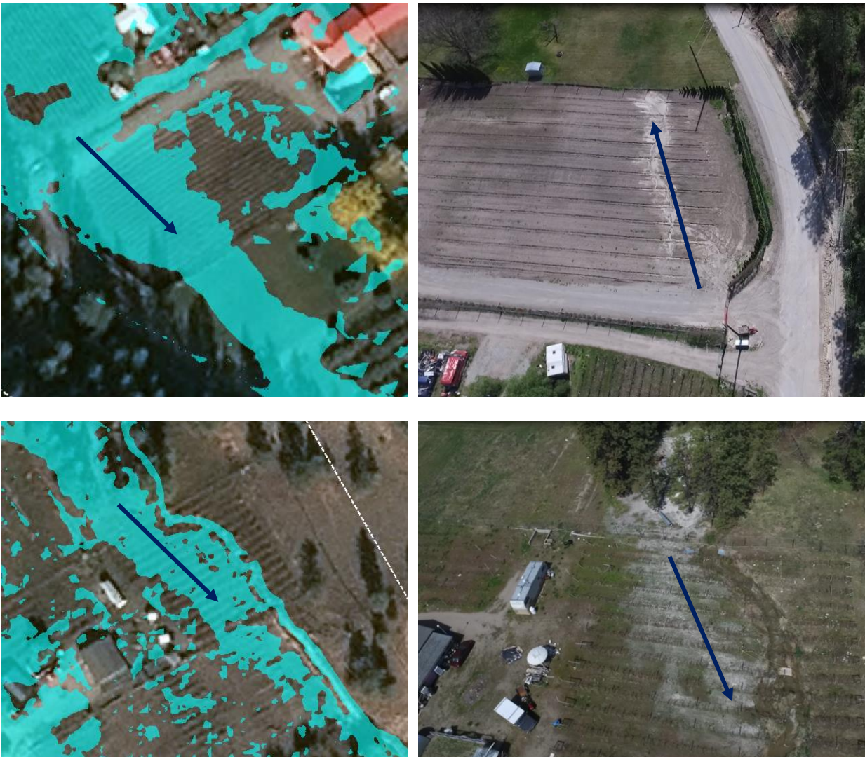
Figure 7.6 Comparison of modelled flow paths with 2018 flood drone footage for Sportsmens Bowl Road area. Top: flooding through fields between Park Rill Creek main channel and Sportsmens Bowl Road. Bottom: flooding through Park Rill Creek old channel alignment.
