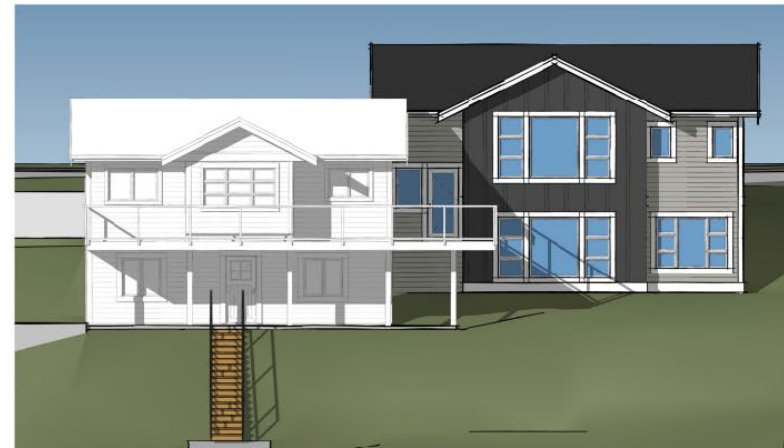
REAR (EAST) ELEVATION 3/16" = 1'-0"
