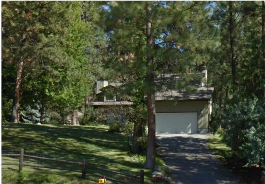
FIGURE 13 An example of good defensible space and low-hazard landscaping solutions in Husula. This combination of a green lawn surrounding the home, as well as no flammable vegetation up against the house, help to significantly lower this home's ignition potential. Although this property does have conifer trees within Zone 1, these trees are well-spaced and pruned and have little chance of candling.
