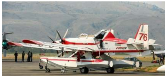
Water-skimmer aircraft—Air Tractor AT-802F—provide critical prepare to support crews on the ground.
