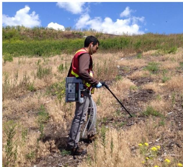
**Photo 7-1 Surface Methane Concentration Scan Using a Portable FID Instrument**
