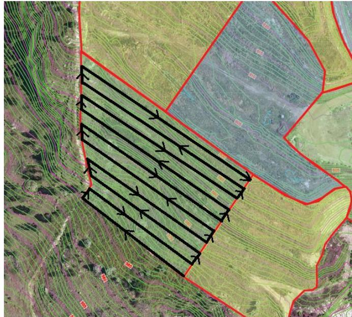
**Figure 7-2 FID Scan Walking Pathway in Grid #1**
