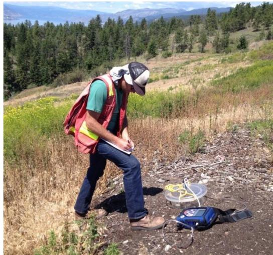
**Photos 7-2 & 7-3 Flux Chamber Test Setup and SHA Staff Conducting the Test at the CML**
