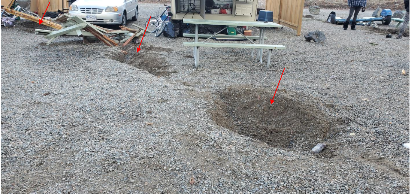
Photo 13 View of ground impact from Rock Fall #1.
