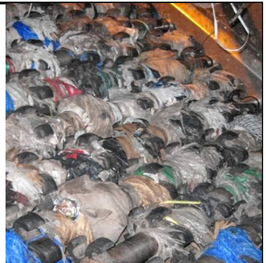
Plastic wrapped around equipment
